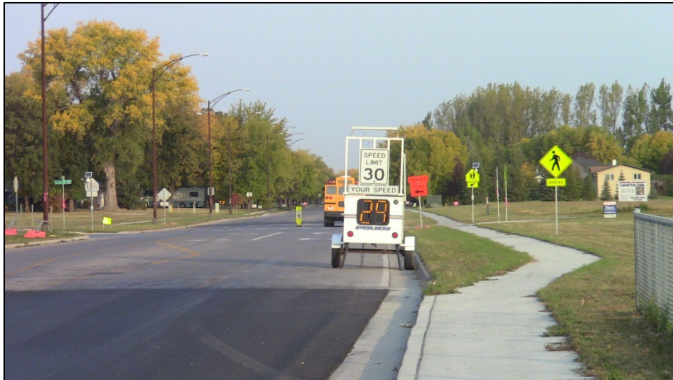
Figure 4.70 Dynamic speed display sign placed inside the traveled way
